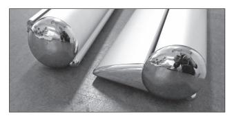
Step 6 Re-attach the end cap by locating and aligning the rear hook. Aim the spring clip into the slot and press to snap in. Ready!
