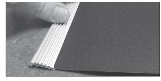
Step 3 Mount the D-profile to the bottom of the graphic. The profile should be applied to the front of the graphic.
