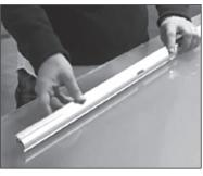
Step 1 Open the Gripper profile. Place it on the table like this.
